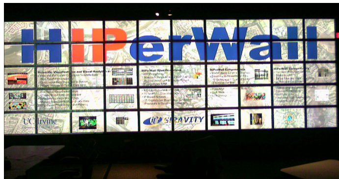
Fig. 3. 200 megapixel tiled display cluster measuring 23 \times 9 ft.
