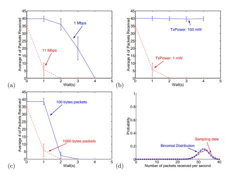
Fig. 2. Reception Range versus (a)data rates, (b)transmitting power, (c)packet size and (d)packet arrival rate distribution
