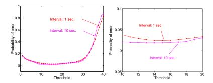
Fig. 5. The probability of error for varying threshold with Data Collecting Interval size of 1 sec and 10 sec.
