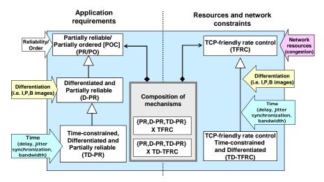
Figure 1: Transport mechanisms to by provided by the QoSTP
