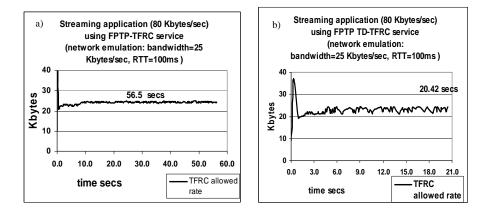
Figure 2: TFRC vs TD-TFRC mechanisms with bandwidth limited to 25 Kbytes/sec
