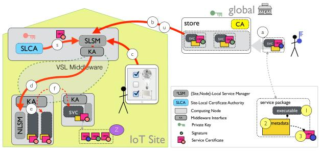
Fig. 2. Proposed Distributed Self-Managing Security Architecture.
