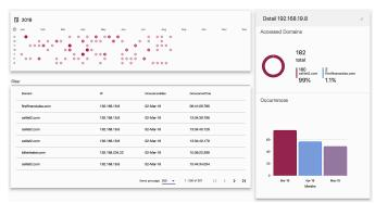
Fig. 2. Operational data view. Components: heatmap calendar view showing the distribution of records based on the domain occurrence (top-left), log details with a search field (bottom-left), IP address inspector (right side) – contains summary of accessed domains for selected IP address (top), occurrence of accessed domains from the selected IP address (bottom).
