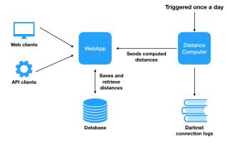
Fig. 2: Architecture of the application
