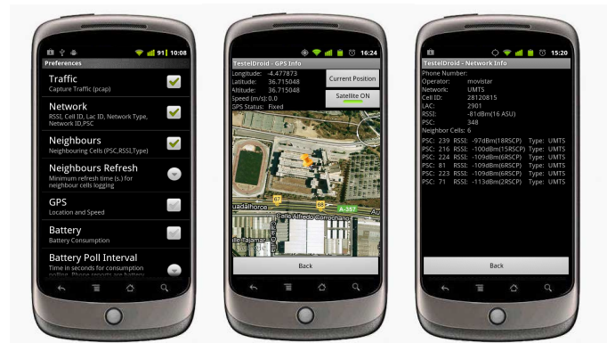
Fig. 1. TestelDroid screenshots, from left to right: Preferences configuration, GPS measurement localization and Network information
