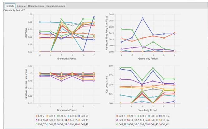
Figure 3. The PM panel showing the KPI statistics of the cells of interest. There are three other tabs between which the operator can switch.
