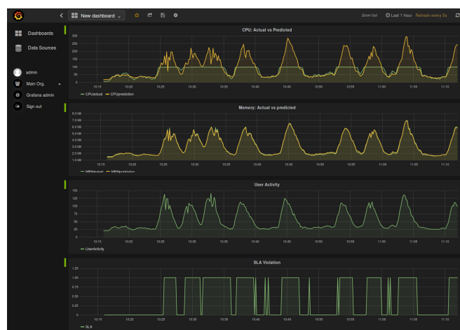
Fig. 3. Predictions for resource needs and actual resource consumption in terms of CPU and memory utilization for a video-streaming service over-time.
