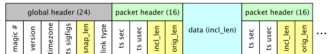
Fig. 1. The record-oriented structure of the PCAP file format. Records and headers are appended sequentially without delimiters or indexing.
