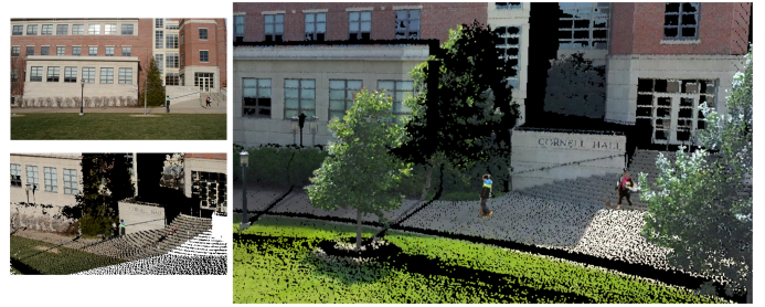
Fig. 2. Creating 3D planes for dynamic objects. Top Left : 2D video frame. Bottom Left : Video frame projected onto range scan without using our method for modeling moving objects. Right : 3D planes constructed for moving objects identified in video using our modeling method.
