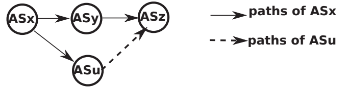
Fig. 5: Example for an alternative route in a trivial AS graph
