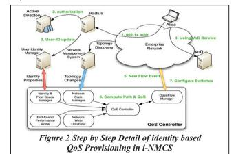
5. **Southbound API**: The i-NMCS framework communicates with the network devices using the Southbound APIs. The fine-grained SDN control is done using OpenFlow protocol. At the same time, SNMP and other traditional
