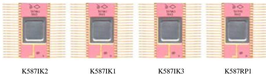
Figure 8. The first in USSR microprocessor complete set, a series K587. It was applied by consumers about twenty-five years.
