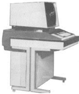
Figure 2. The device of visual display (UVO). The symbolical display. Diagonal of the screen (43 cm); Size of the screen (220x200 mm); Symbols (up to 2048); Lines on the screen (32); Symbols in line (64); Size of a symbol (3.5x2.5 mm); Ensemble of symbols (128).
