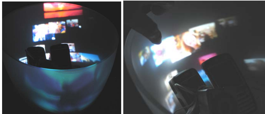
Figure 3. Bowl sketch built using projection system and translucent glass bowl.
