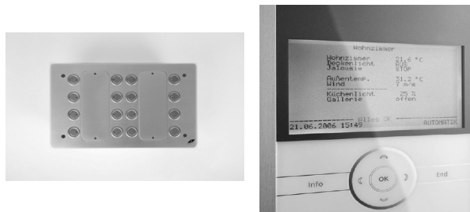
Fig. 2. Examples of smart home switching components (sources: http://www.moeller.at , http://www.eib-home.de/gepro_knx-eib-tableau_2006.htm , 2007-03-17)
