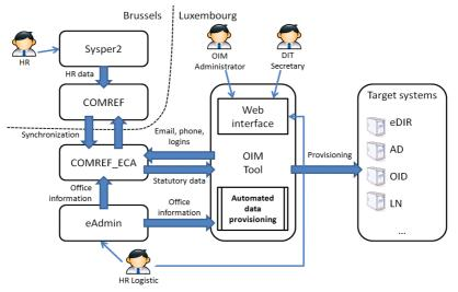
Fig. 4. Overview of the ECA OIM architecture
