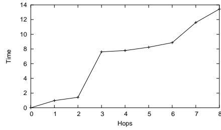
Fig. 3. Inquiry-oriented approach elapsed times
