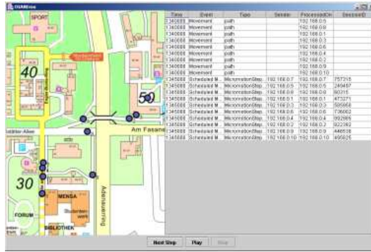
Fig. 4. Simulator DIANEmu View. Left: Visualization of users moving on campus. Right: Message view of the underlying meta protocols.
