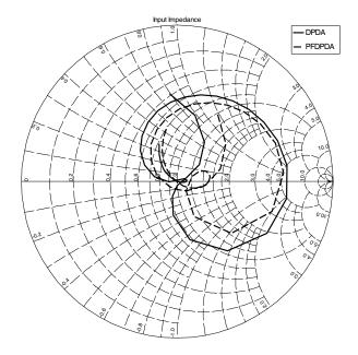
Fig. 4. Return Losses of DPDA and PF-DPDA
