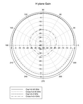
Fig. 6. Gain Pattern of PF-DPDA Antenna
