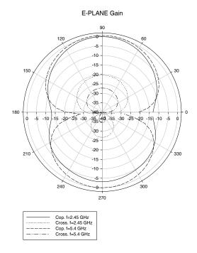
${\bf Fig.\,5.}$ Gain Pattern of PF-DPDA Antenna
