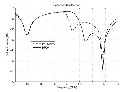
Fig. 3. Return Losses of DPDA and PF-DPDA
