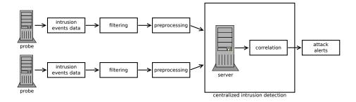
**Fig. 1.** Intrusion detection with centralized collection and correlation of data from various probes. Every piece of information is sent to a server which handles the correlation.
