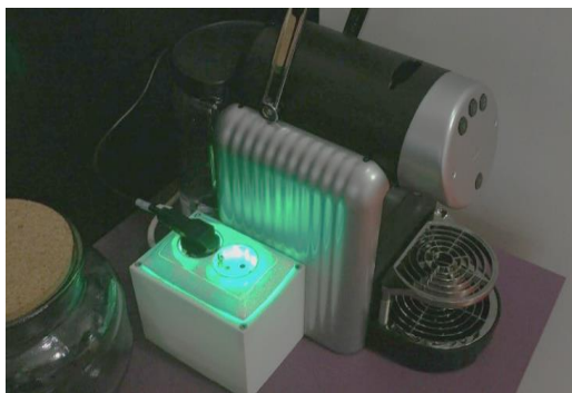
Fig. 2. Wattapp as it was deployed next to the coffee machine, in this particular case the consumption is very low.
