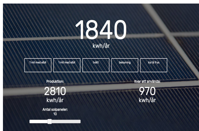
Fig. 1. The computer interface showing consumption in the top (1840 kwh/year), the active blocks as boxes, production in the bottom left (2810 kwh/year for 10 solar panels) and how much is left to use (970 kwh/year).
