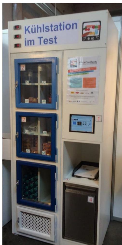
Fig. 1. Cooling station prototype (1: tablet, 2: windows of refrigerator, 4: waste paper basket); “Kühlstation im Test” means “Test of a Cooling Station”
