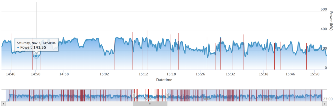
Fig. 6. Weekly consumption of the TV # 4 with the TV Box and Home Cinema, showing how the the noise in the signal increases the number of false detections.
