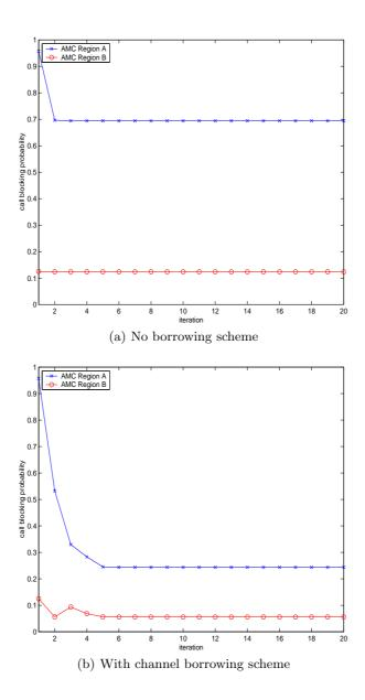
Fig. 6. Blocking probability using channel borrowing scheme with  $\rho = 5$
