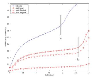
Fig. 4. Blocking probability (AMC vs No AMC.)
