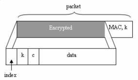
Fig. 2. Packet Structure
