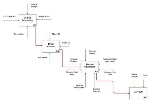
Fig. 1 IDEF0 of the dismantling at WR.
