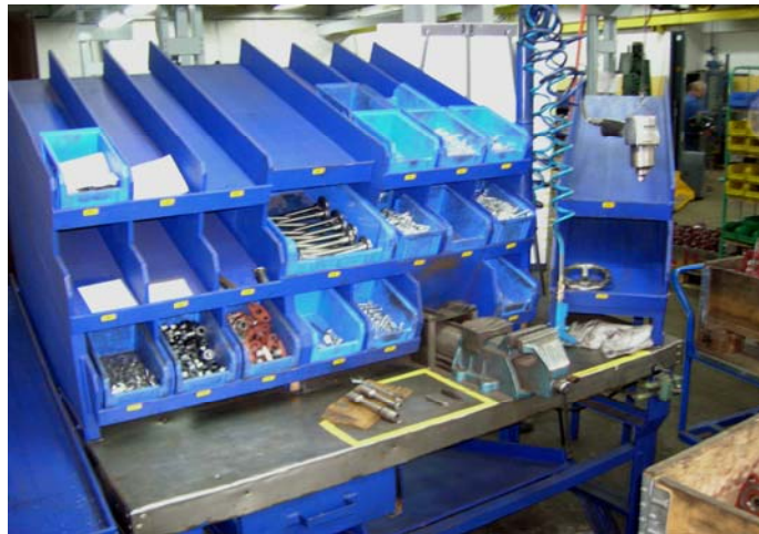
Fig. 3. Flow rack for material presentation within assembly cell
