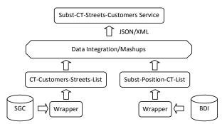
Fig. 3. Distributor's service integration for substation-customer.
