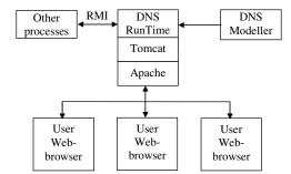
Figure 3 DNS software architecture
