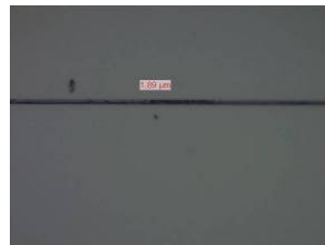
Fig. 8. : Adhesive gap of < 3 \mu\text{m}
