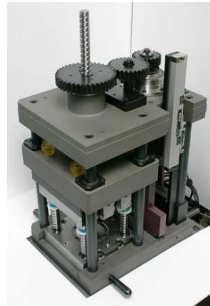
Fig. 4. CAD model of desktop forming system Fig. 5. Manufactured desktop forming system
