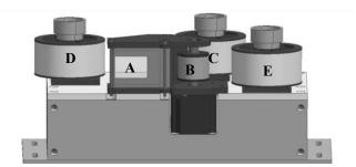
**Fig. 5.** The tape feeding system supplies adhesive gaskets automatically. Gaskets are provided on foil rolls and are covered by protection foils. Before hybrid bonding, one gasket is moved to the joining area while the protection foil is removed.
