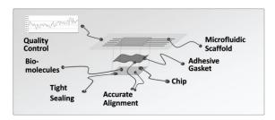
Fig. 1. Components of micro fluidic cartridge
