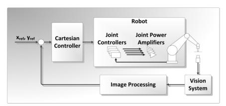
**Fig. 6.** Look-and-move control loop: a vision system provides exact information about gasket position. The robot aligns the chip to the adhesive gasket before hybrid bonding.
