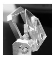
Fig. 4. Chip Inspection Cradle
