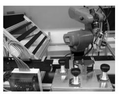
**Fig. 2.** The robotic cell includes an articulated robot (middle), two supply systems for chips and scaffolds (left and right of the robot), a feeding system for adhesive gaskets (front) and a sealing test module (front left).
