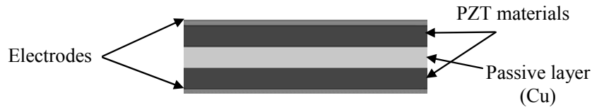
Fig. 3. Bending cantilever structure
