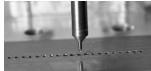
Fig. 11. Extraction of a ball out of the mesh with the capillary gripper
