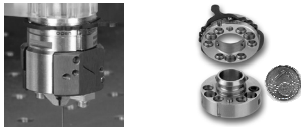
Fig. 2. Left: Endeffector: Parallel Micro Gripper (with integrated standardised interface) Right: Micro Tool Change System
