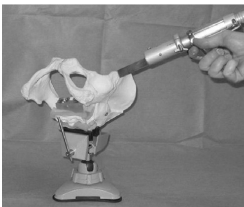
Fig. 2. The sawbone is rigidly fixed by a steel clamp with a 360°-rotational base. The cutting is performed using an oscillating saw.
