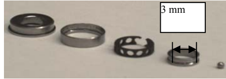
Fig. 6. Spin Bearing Assembly Components
