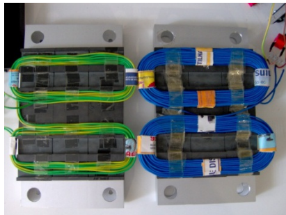
Fig. 14. Secondary and primary windings respectively in yellow/green and blue
