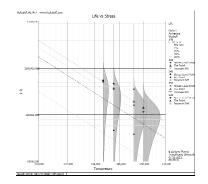
**Fig. 5.** Life vs. Stress for profile S1 (temperatures: 338 K, 343 K, 353 K, 358 K) and the duty rating stress level 348 K.
