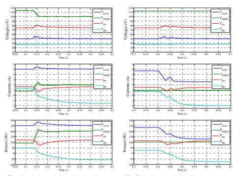
**Fig. 6.** Load, generator, PV and battery voltages, currents and powers during a PMSG transient.
