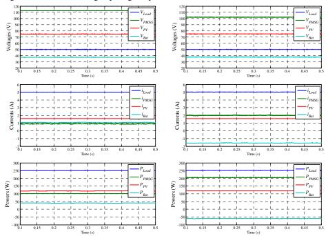
Fig. 4. Load, generator, PV and battery voltages, currents and powers for a PMSG load torque equivalent to 17% of the rated torque.
