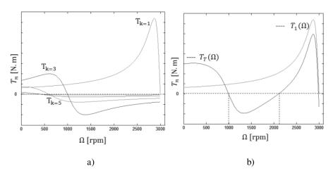
**Fig. 6.** a) Individual contribution of the main harmonics to the resulting torque. b) Resulting torque as a function of speed.
