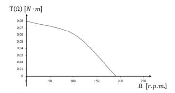
Fig. 9. Experimental torque/speed characteristic for topology T1.
