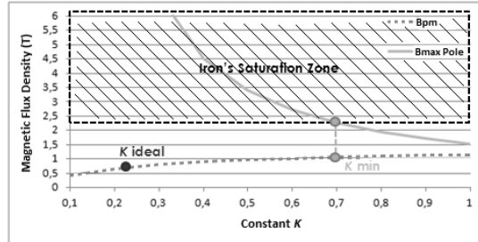
Fig. 3. Magnetic flux density with the variation of K .
