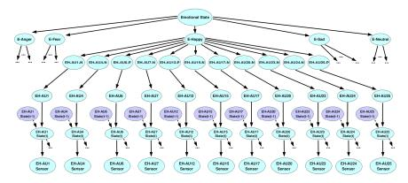
**Fig. 3.** Dynamic Bayesian Network (DBN) - partial structure. Light nodes are of the present time slice, while dark nodes belong to the previous one (t-1). The dashed arrows connect nodes of different time slices: from past to present and from here to future (these nodes are not represented).
