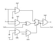
Fig. 4. Data path bit slice structure.
