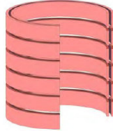
Fig.2. Multi-layer coils carrying the same or different current in each layer. The proximity of the tapes in the same position of consecutive layers makes the AC loss different from in a single layer coil.
