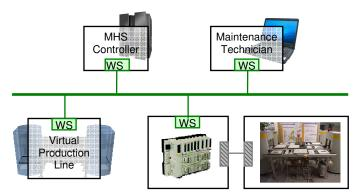
Fig. 2. Virtual SoA-based production system with hardware in the middle.
