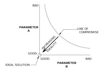
As we try to improve one parameter (material removal rate) the other (machining time) becomes worse, and vice versa. It would appear that we are constrained to remain on line of compromise curve, which defines the set of possible compromise solutions available to us. What we would like to able to do is to move off the line of compromise curve to a more ideal solution – i.e. in the direction shown by the dark arrow. To achieve this we need to find a way of resolving the contradiction.
