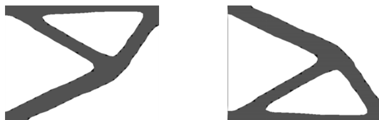
Fig. 4. Topologies resulting from the mono-objective optimizations: optimal density distributions under boundary conditions 1 (left) and 2 (right). The objective function is the minimal deformation energy under a maximum mass constraint of 3 kg.
